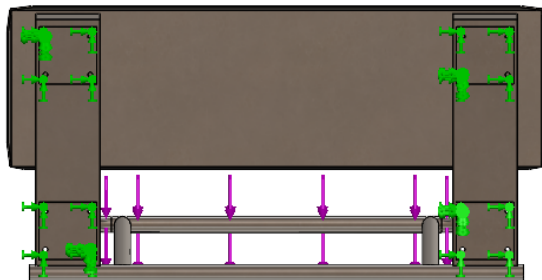
Fig. 21. Force Conditions of Finite Element Analysis.
