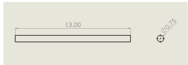
Fig. 33. Axes 1 of 13 inches with radius of 3/4.
