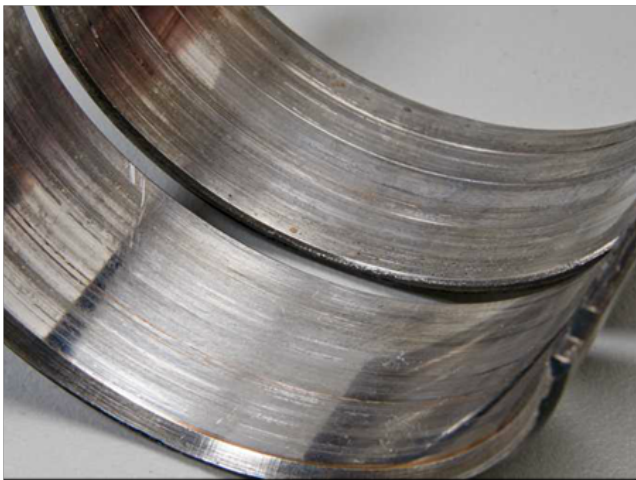
Fig. 35. Wear due to small particles in bearings.
